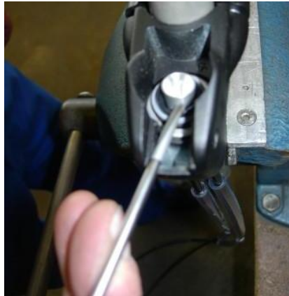
Figure 64: Removing the aluminium cup
