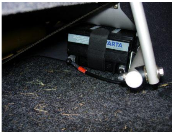
Figure 32: On-board battery C42 / C42B / C42C / C42E
