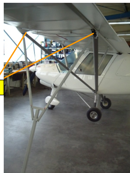
Figure 86: Jacking up the main landing gear with a Kny fork
