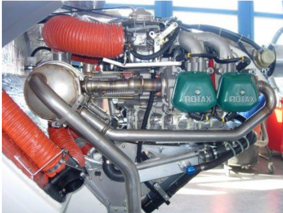
Figure 22: Rotax 912ULS engine (C42B / C42B UK / C42C / C42E)
