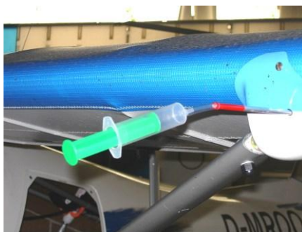
Figure 76: Checking the pitot pressure system
