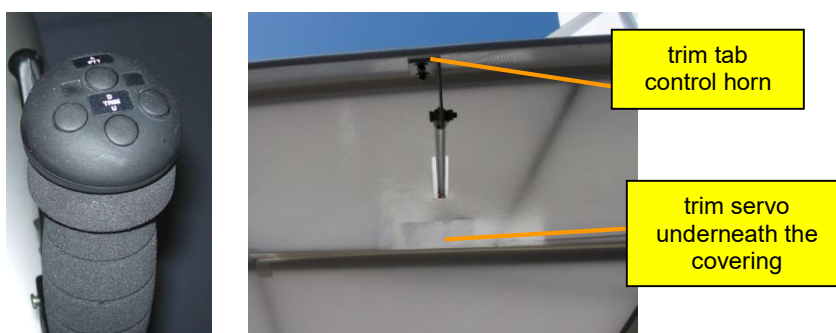
Figure 38: Activation of the electrical trim tab
