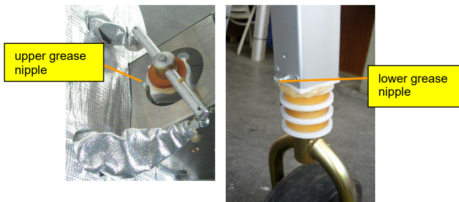
Figure 61: Grease nipples, nose wheel landing gear
