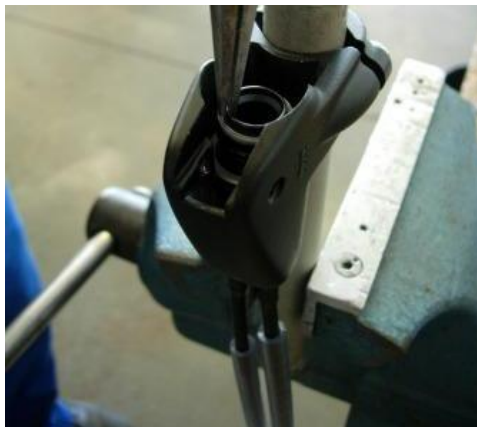
Figure 65: Removing the pressure piston
