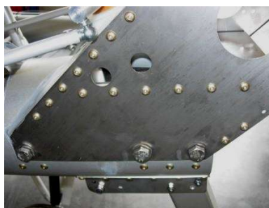
Figure 55: Rivet connections on the engine mount
