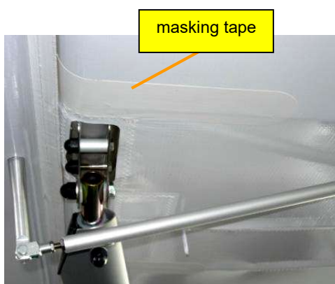
Figure 67: Batten covering on the wing underside
