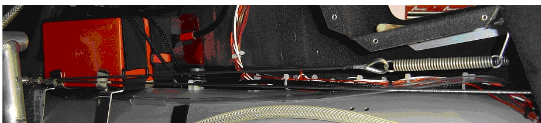
Figure 43: Rudder return cable & spring for C42B UK / C42 E
