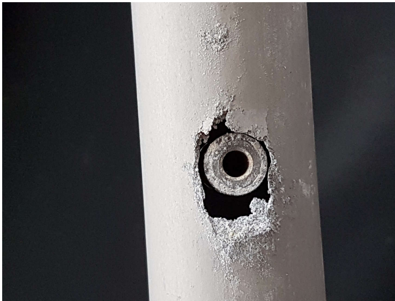
Figure 1, severely corroded aileron centre eyebolt hinge attachment point (hidden under fabric covering in service).
