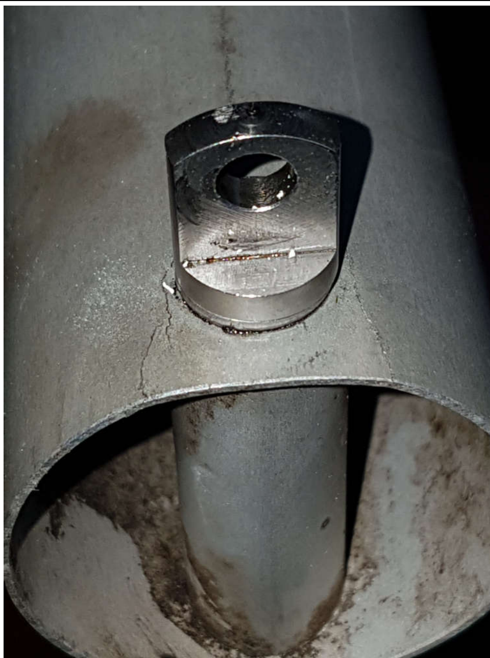
Figure 2, cracked aileron inboard eyebolt attachment, caused by overtightening eyebolt onto flat ended insert (not hidden by fabric covering in service).
