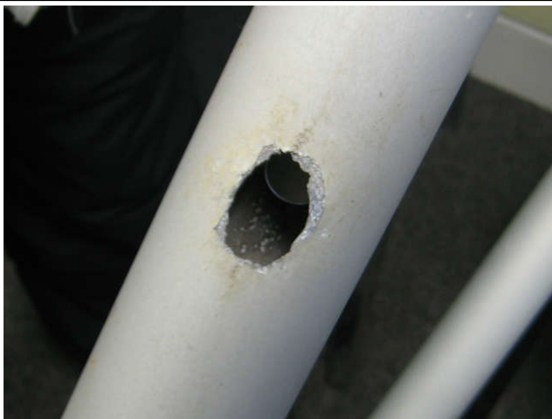
Figure 3, hole where aileron horn passes out lower side of aileron front spar tube (hidden beneath fabric covering in service).
