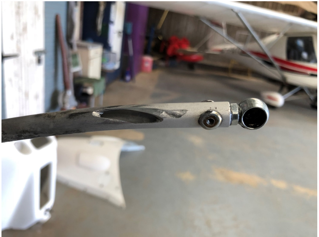
Figure 1, severely abraded port-side nosewheel steering pushrod.
