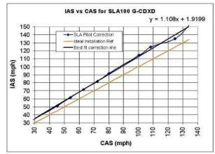
To use the graph to correct for the pitot-static installation errors find the IAS along the vertical axis and move across the graph to find the intercept with the back line; the CAS can then be read off of the horizontal axis.
