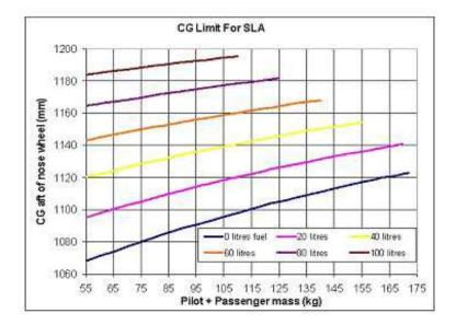
Pilots should be aware that stick forces and displacements will become lighter with aft CG (typically a heavy crew and full fuel) and heavier with forward CG (typically low fuel, light pilot only). In addition, at aft Cg, the stability will be reduced and as a consequence the aircraft will have less tendency to return to the stable condition when in, for example, turbulent conditions.
