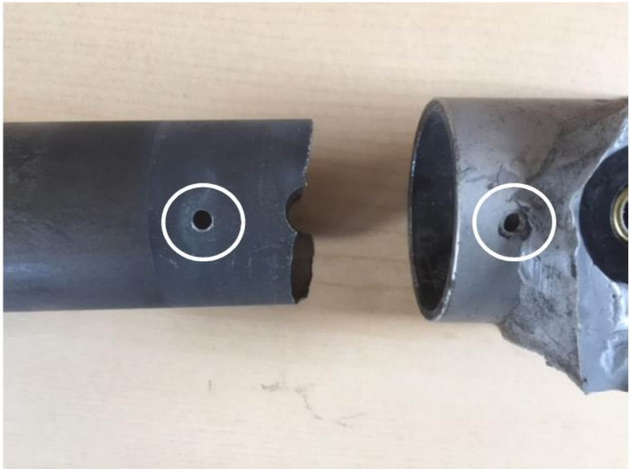
Figure 2 - Failed A-strut removed from outer sleeve part on right of picture. Circled holes show location of the rivet which was holding the parts together.
