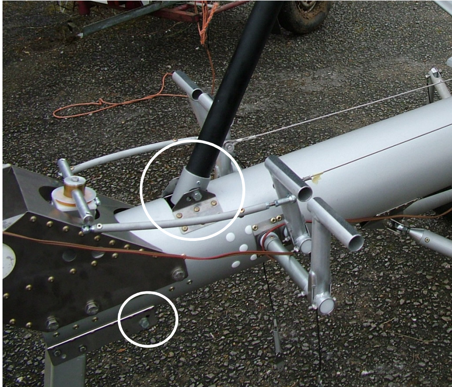
Figure 1; A-strut attachment to upper surface of main fuselage tube. Lower attachment bolt visible beneath main fuselage tube at aft end of bracket attached to nose leg.
