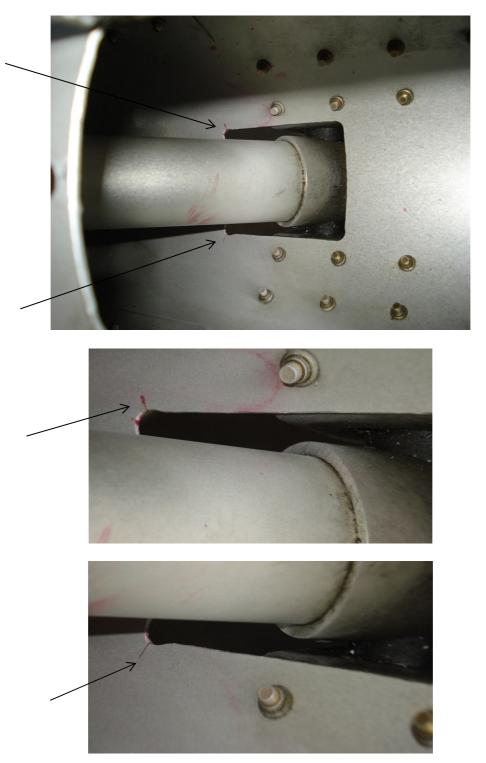
Example cracks on lower surface of main fuselage tubeat corners around A-strut cut-out.
