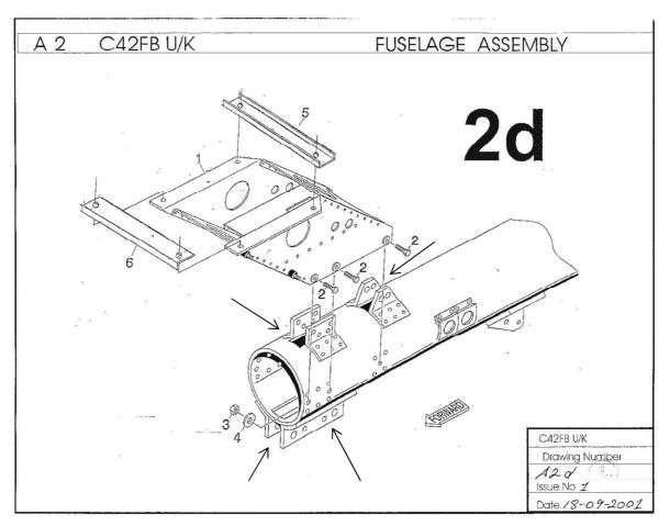
Nose-leg and A-strut cut-outs at front of main fuselage tube in vicinity of engine mount.
