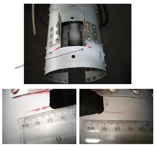
Example cracks on upper surface of main fuselage tube at corners around nose-leg cut-out.
