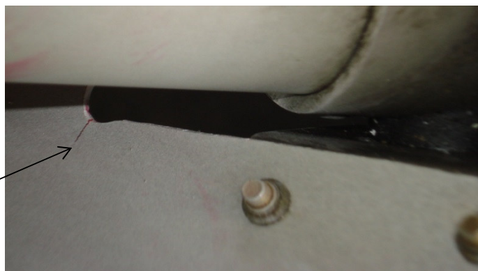
Example cracks on lower surface of main fuselage tube at corners around A-strut cut-out.
