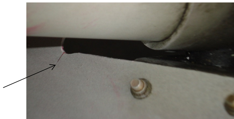
Example cracks on lower surface of main fuselage tube at corners around A-strut cut-out.
