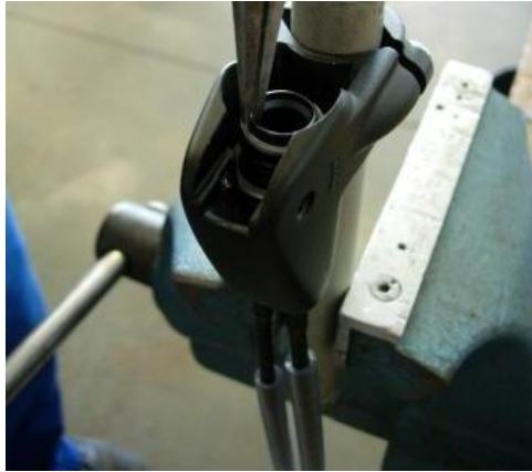
Figure 64: Removing the pressure piston
