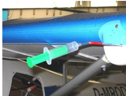
Figure 75: Checking the pitot pressure system
