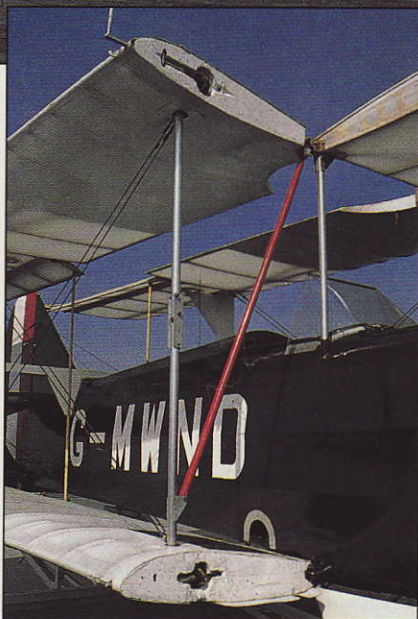
The wings fold for quick and easy trailering. Straight braces (painted red) are used to support the folded wings.
