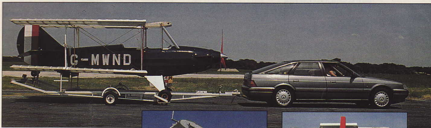
The wings fold for quick and easy trailering. Straight braces (painted red) are used to support the folded wings.
