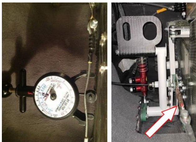
Figure 3-14 Adjustment on turnbuckles to reach required tension
