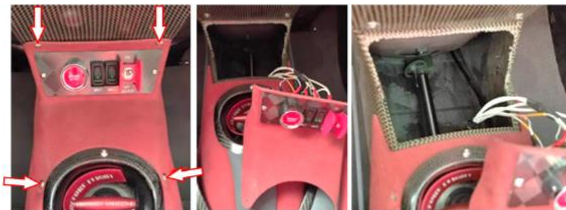
Figure 4-39 Remove fairing in front of rear seat
