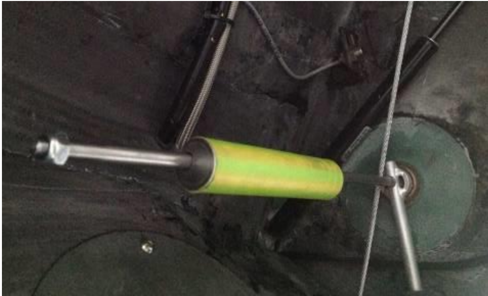
Figure 3-7 Reverse hammer used to remove wing pins
