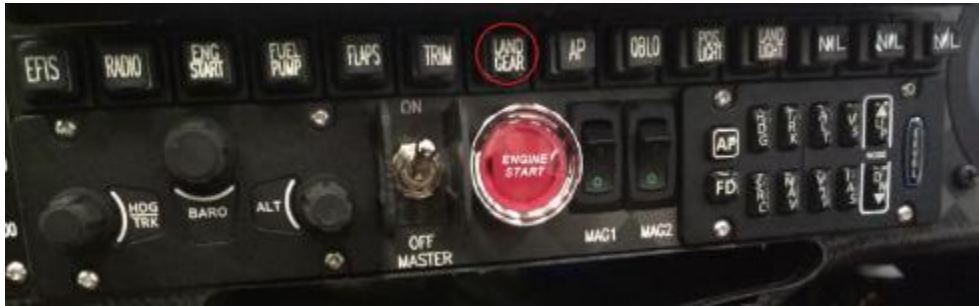
Figure 4-13 Landing gear circuit breaker OFF
