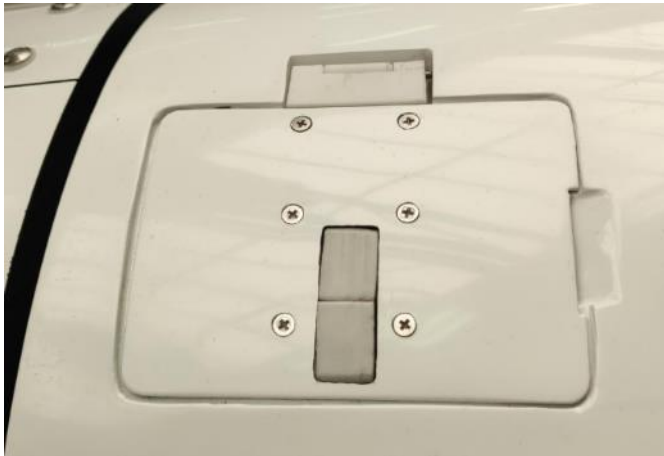
Figure 3-55 Movable ballast engine compartment - in baggage compartment
