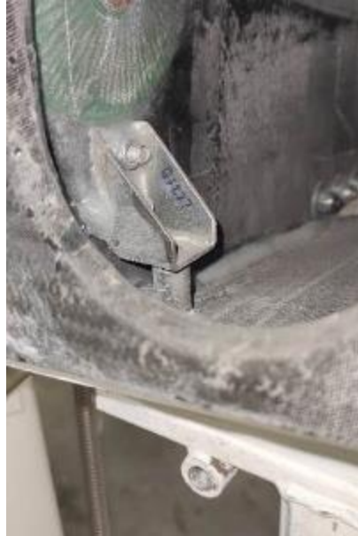
Figure 4-4 Welded bracket for airplane lifting
