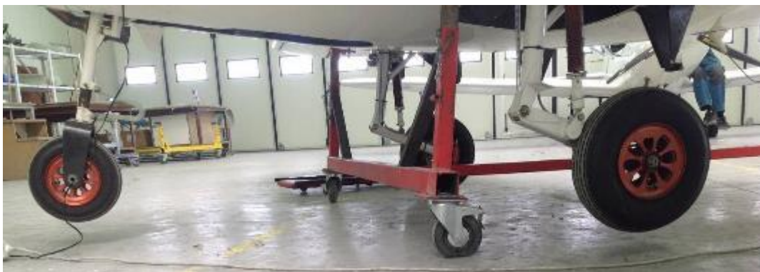
Figure 4-12 Example of airplane on trestle-stand
