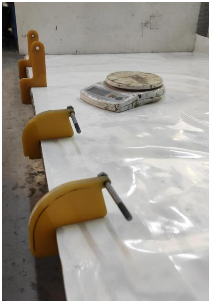
Figure 3-52 Tools for weight and static moment determination
