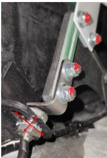
Figure 4-35 Sensor adjustment, example on nose landing gear
