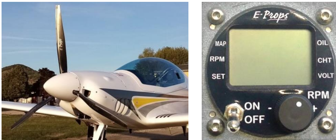
Figure 2-40 E-prop Glorieuse and constant speed unit
