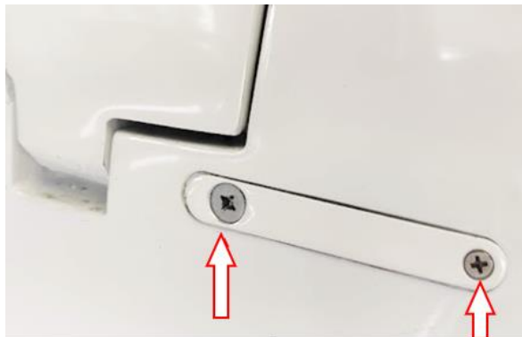
Figure 3-41 Remove hinge cover
