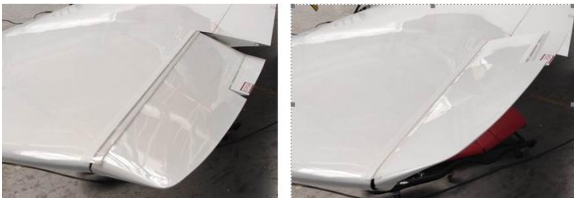
Figure 2-9 Automatic tabs on aileron
