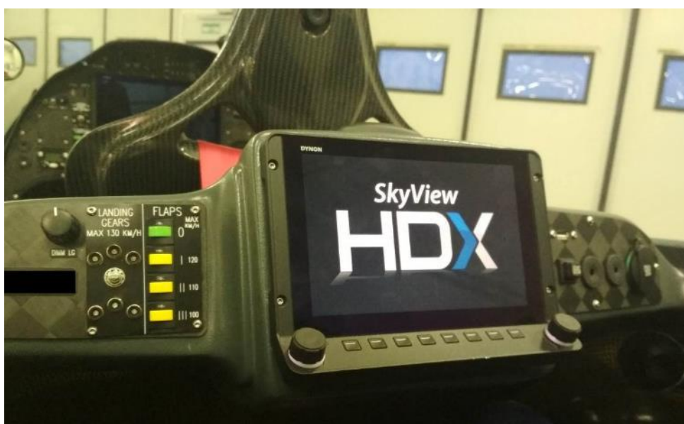
Figure 2-35 Rear instrument panel Dynon SKYVIEW
