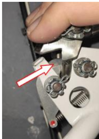
Figure 4-29 Checking of locked rod eye
