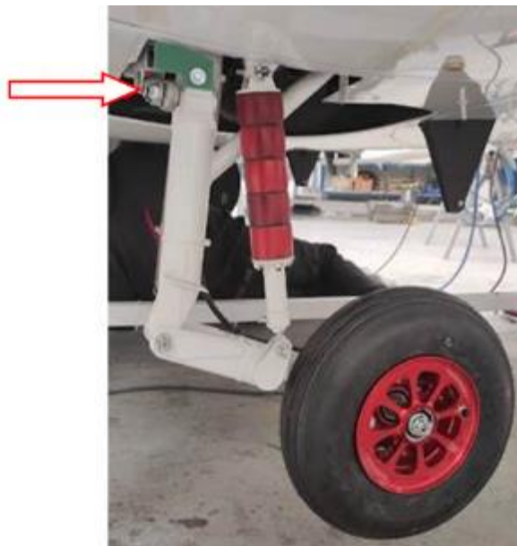
Figure 4-33 Ball bearing to adjust vertical position
