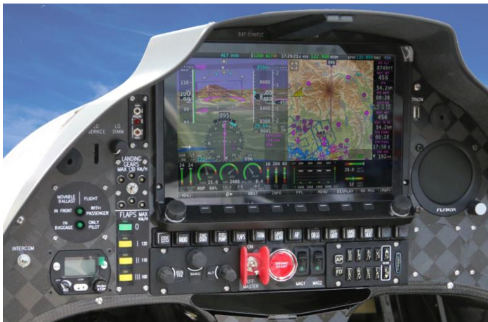
Figure 2-33 Example front instrument panel with DYNON SKYVIEW HDX
