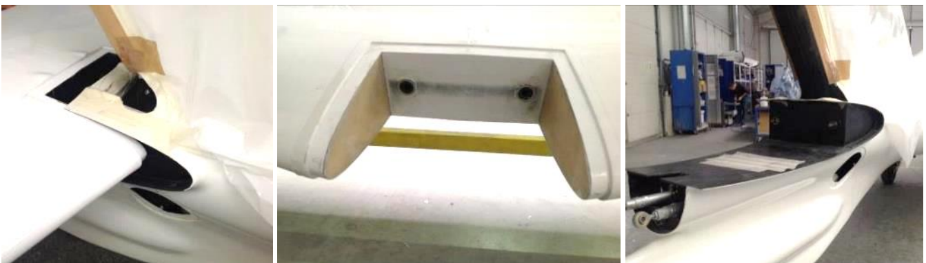
Figure 3-10 Horizontal tail unit removal example
