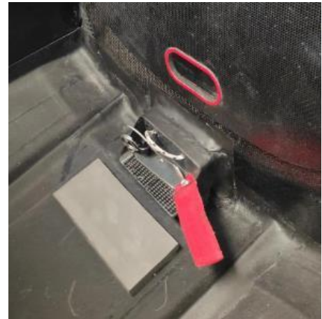
Figure 3-55 Movable ballast engine compartment - in baggage compartment
