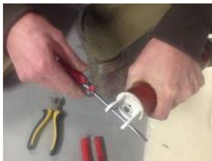
Figure 4-44 Remove upper bracket
