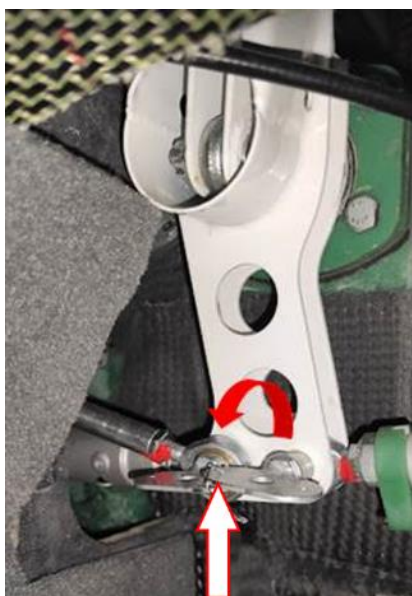
Figure 3-1 Disconnect butterfly bolt
