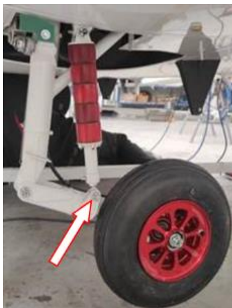
Figure 4-34 Ball bearing to adjust shock absorber length
