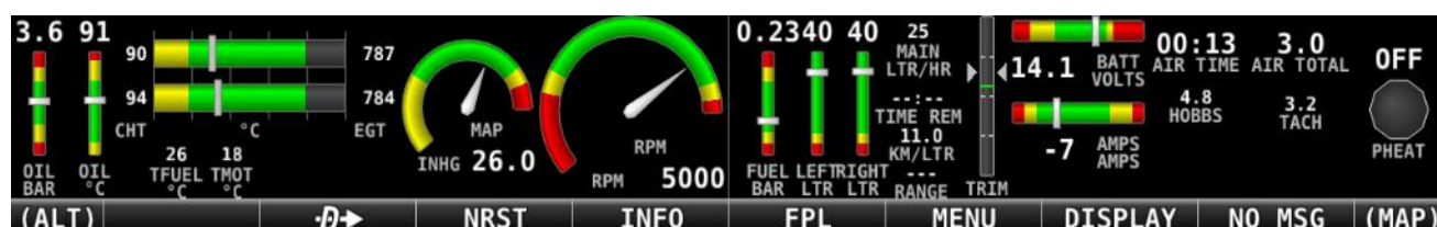
Figure 2-37 example of Dynon SkyView engine parameter
