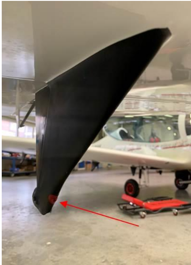
Figure 2-31 Fuel tank air vent
