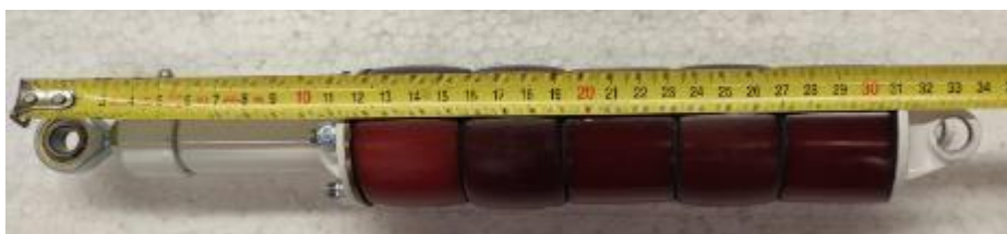
Figure 4-42 Shock absorber nominal length
