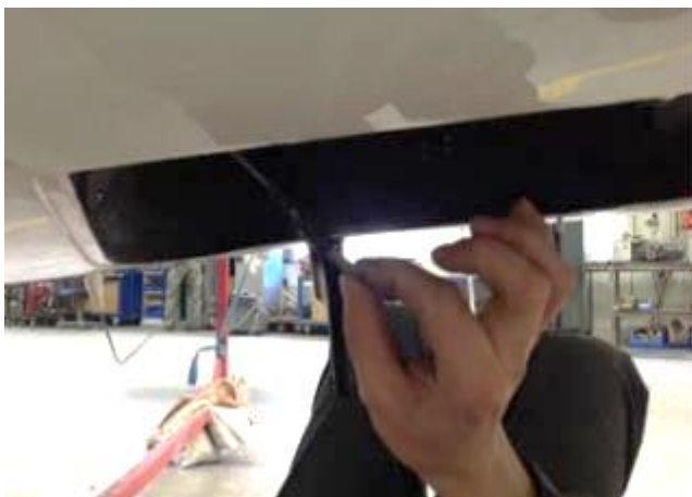
Figure 4-15 Catching the wire- view from the front and from the rear
