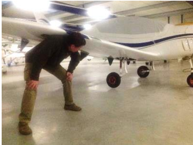
Figure 4-10 Airplane lifted with operator below main spar
