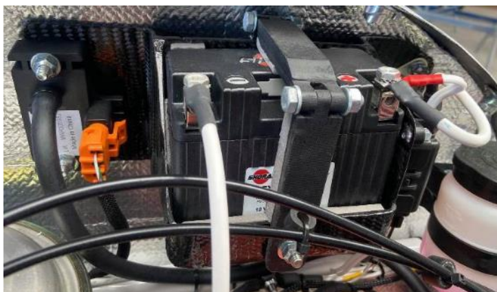
Figure 2-29 Battery SHORAI LFX L2-BS installed on SHARK
