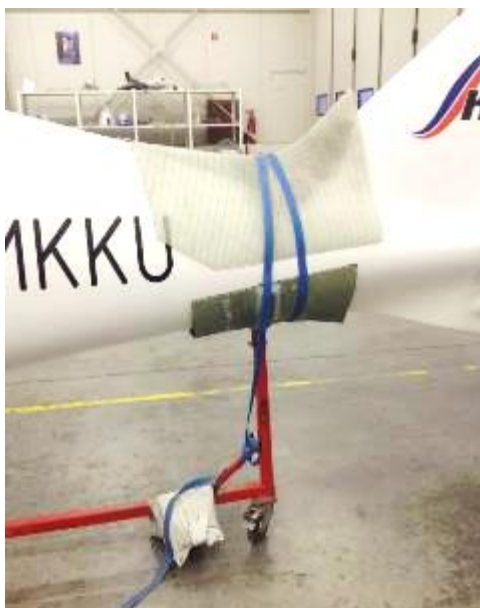
Figure 4-6 Tail cover for airplane lifting
