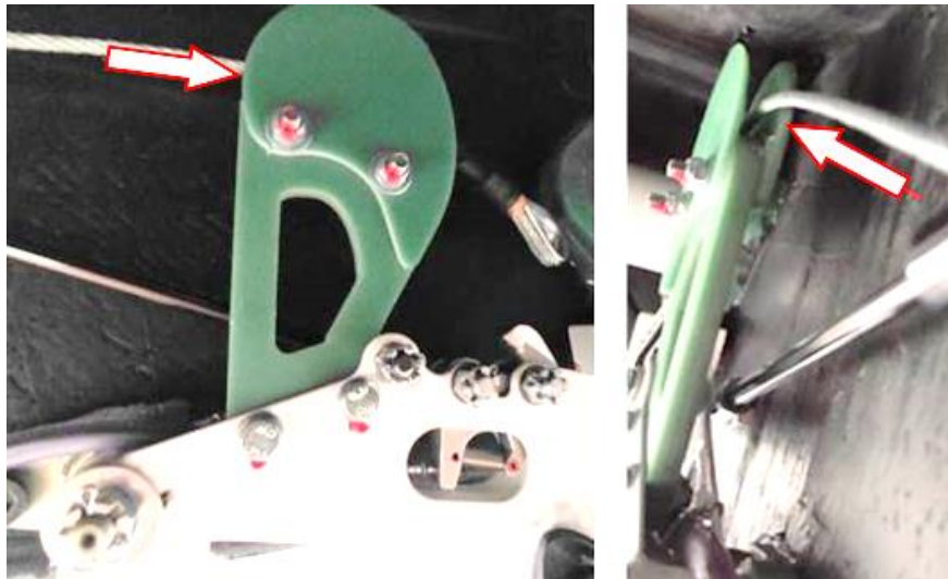
Figure 4-20 Wire must go via pulley
