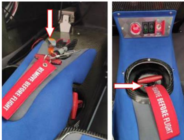
Figure 3-26 Lock activation handle
