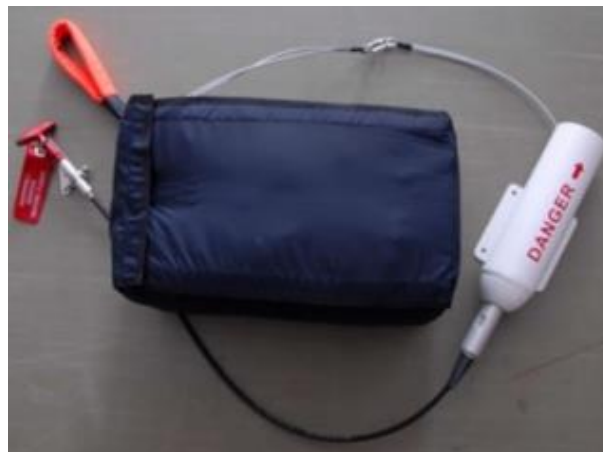
Figure 2-48 Parachute case with rocket
