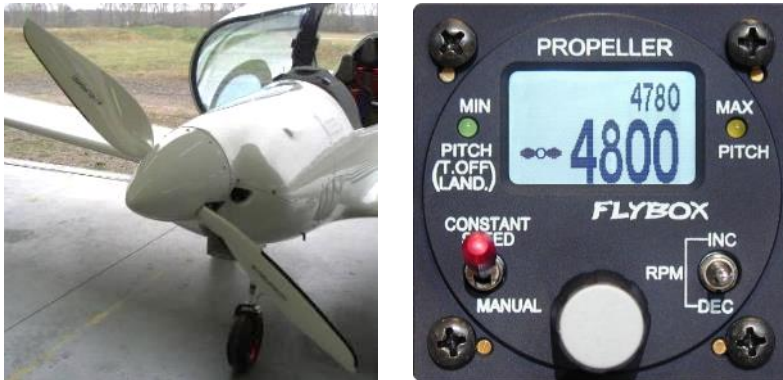
Figure 2-39 Neuform TXR2-V-70 and constant speed unit
