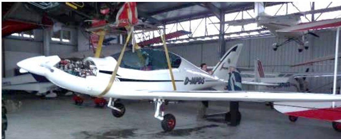
Figure 4-9 Airplane lifted with belts
