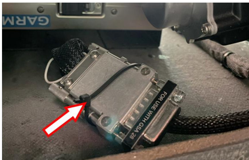
Figure 3-48 secure connector by a cable tie
