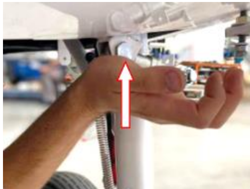
Figure 4-30 Push locking strut
