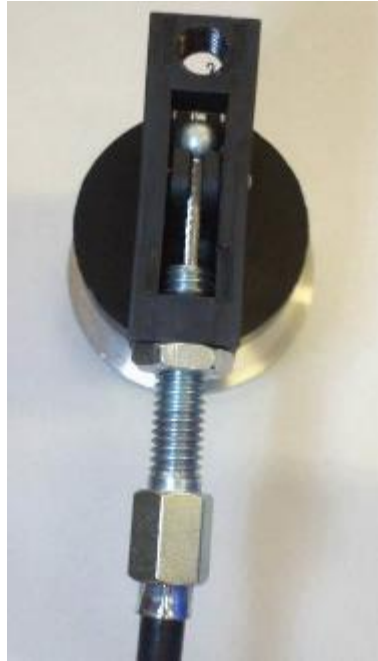
Figure 4-53 Correct position of bowden end
