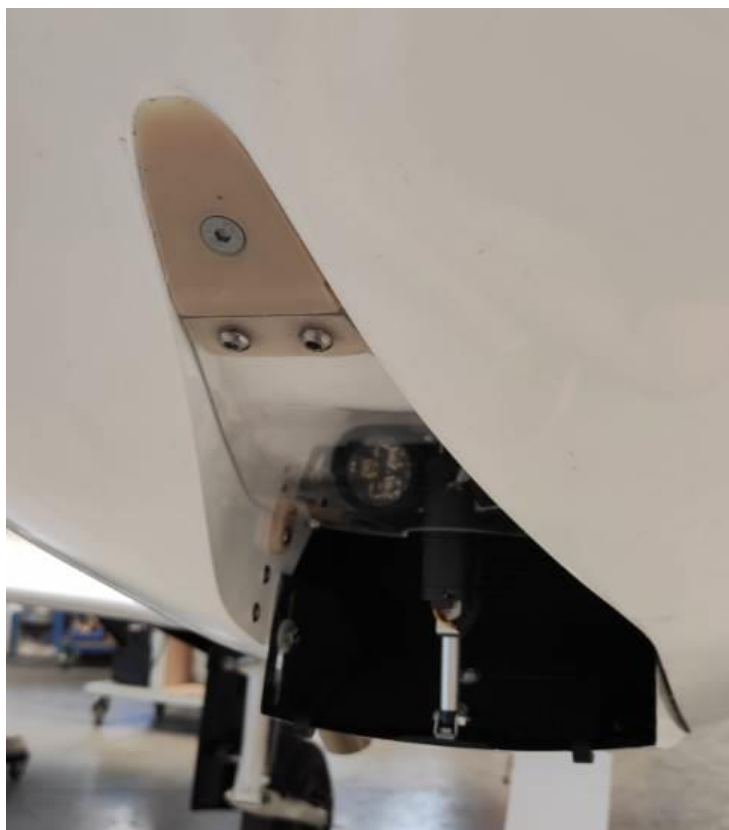
Figure 2-44 Air intake regulated by servo
