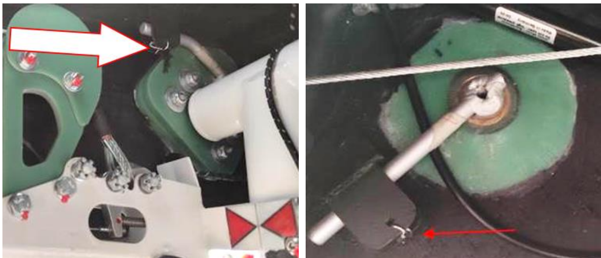
Figure 3-6. Cut safety wire from wing pins
