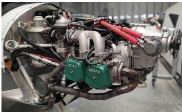
Figure 2-36 Rotax 912 ULS installed on SHARK
