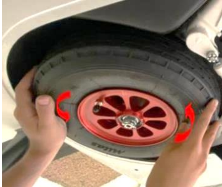
Figure 4-32 Rotate wheel to check eventual contact
