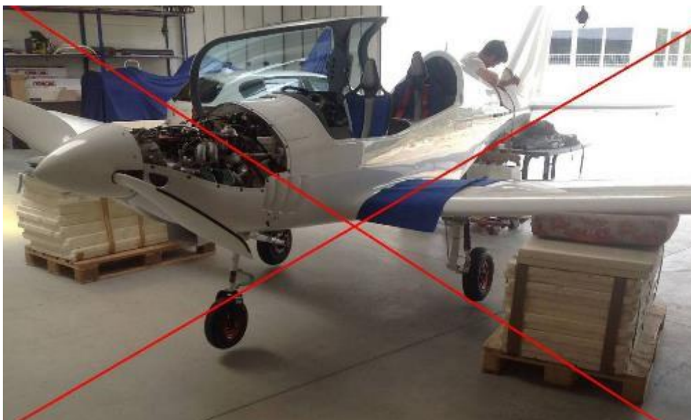
Figure 4-11 Do not use hard block below wing
