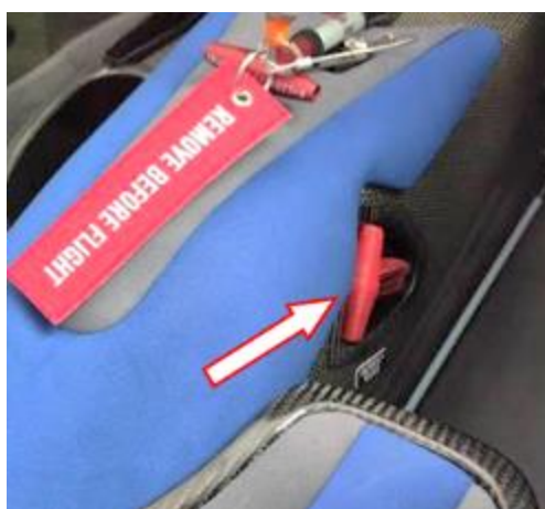
Figure 4-23 Emergency release handle
