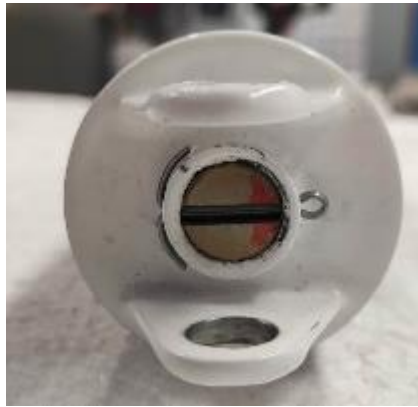
Figure 4-43 Remove cotter pin
