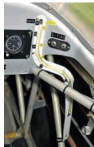
In typical microlight style, fuel level is indicated by a sight tube, in this case in the front cockpit (but clearly visible to the pilot flying solo from the back seat)
