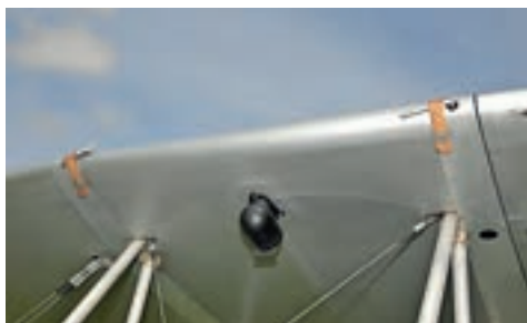
1 As with the 1920s Gipsy Moth, the Ranger's folding wings are secured by pins held in place by leather straps, visible here, either side of the centre section...
