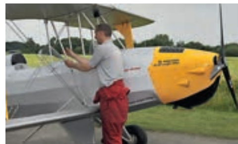
2 ... Before the wings can be unlatched jury struts must be fitted, to maintain the shape of the wing cellule and tension on the bracing wires...
