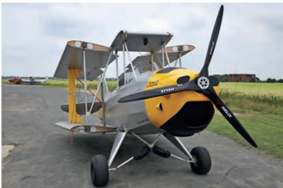
5 ... And, with wings folded, the Ranger's modest span is reduced by two-thirds, from 7m to 2.3m. We reckon your base airfield really should offer a proportional reduction in hangarage fees!
