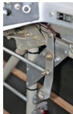
... and the matching 'upside down' trim lever on the starboard side. Bonus points here for proper manual operation, rather than electric trim
