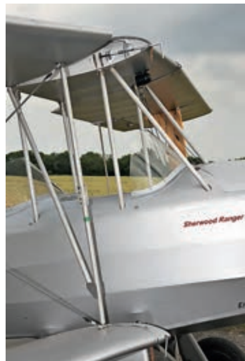
4 ... With the jury struts and stay braces fitted, the wings are unlatched and folded back – a quick and easy one-man job...
