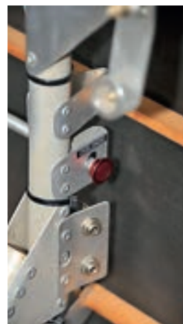
With just the one main tank, a simple on/off fuel valve is all that is required, operated by a pushrod tipped with a red knob
