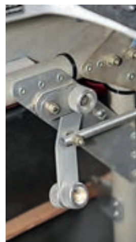
The strange - but effective - 'upside down' throttle lever, complete with nicely machined hand grips and friction adjustment knob...
