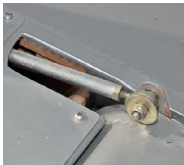
Rod-operated control surfaces, almost free of friction and always more positive in feel than cables, help in providing the Ranger's notably 'taut and crisp' handling
