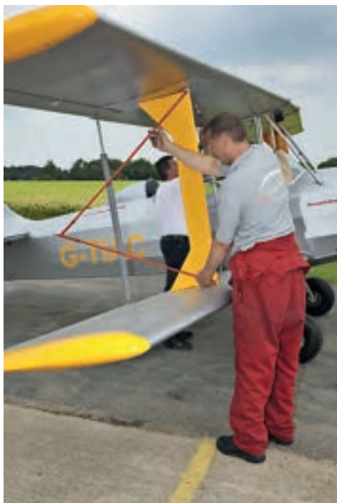
3 ... Next, stays are fitted to the interplane struts. These latch on to the fuselage and brace the folded wings for storage or transport...
