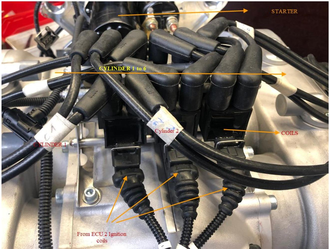
The spark plug cables (with spark plug cable heads) are fixed on the ignition coil stand and grouped by two. (See figure above).
